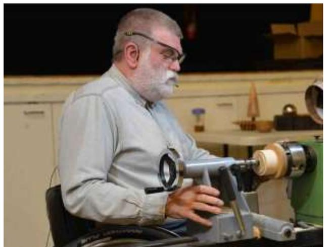
corner each time, then starts at the other corner and does the same again until closer to round. This means that any cracks in the wood do not splinter out like would happen if you roughed the wood down from one end to the other. As wood gets closer to round Chris changes the cut slightly to “float” the bevel and get a better finish.
