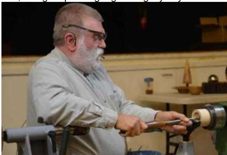
by pushing and wiggling tool in circular motion, said the wiggling ensures the drill hole is just bigger than the gouge so it doesn't bind in the hole. Chris pointed out that stability is the key when doing this and said he rests his elbow on the tail stock to help with stability. Chris then widens the hollow to size with a scooping out motion with the tip of the spindle gouge. As it gets to near the correct size he transitions from the scooping cut, to cut the bottom, to a lower wing sheer
