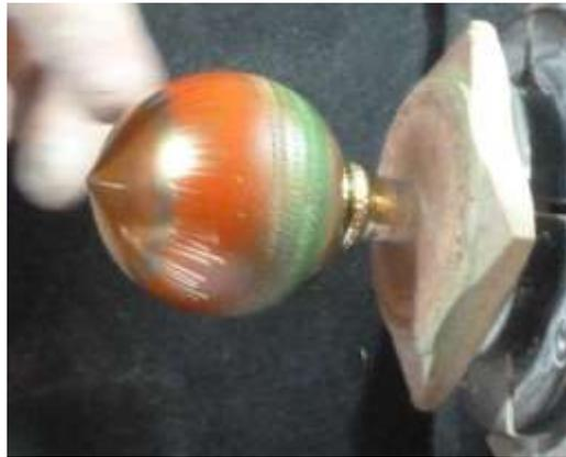
The green and red were sprayed lightly with the lathe turning. The gold was sprayed on the top and bottom of the bauble with the lathe running fast to allow the paint to run up and down the piece to towards the middle.
