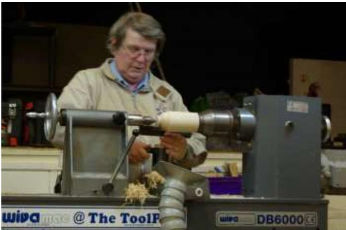
the inside could be sanded and finished as desired. Tony indicated that the outside of the egg would later be painted, hence the lack of concern over the grain or bland featuring of the timber. So if desired the inside of the egg could either be painted or polished.
