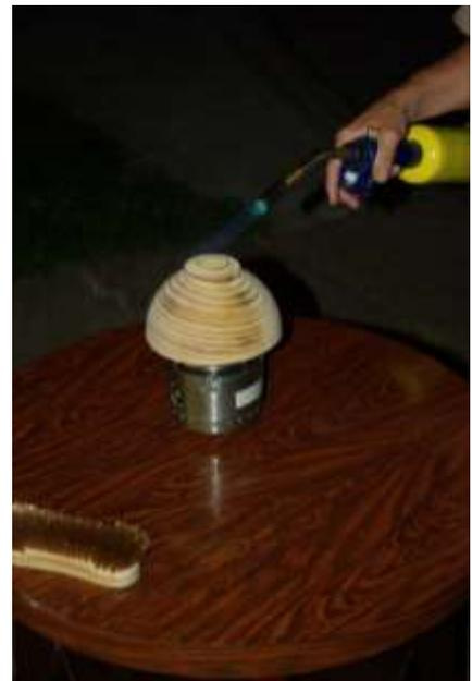
After spraying it would be necessary to leave the blank to dry for a minimum of one hour but preferably overnight. For the purposes of this evening's demonstration Mary performed a quick Blue Peter moment and mounted a blank she had previously prepared to this stage.
