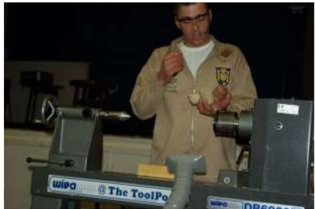
Smooth cylinder achieved Richard examined the outside to decide top and bottom. With Pine, and other wood, there is always a risk of knot ingress. These features need to be carefully incorporated into the final design. In this case the knots location would have coincided with the Bill towards the top of the stem, which could at worst have risked break-out and at least be unsightly. If placed at the lower end it aligned with widest part of the stem, which was deemed to be the lesser of all evils.
