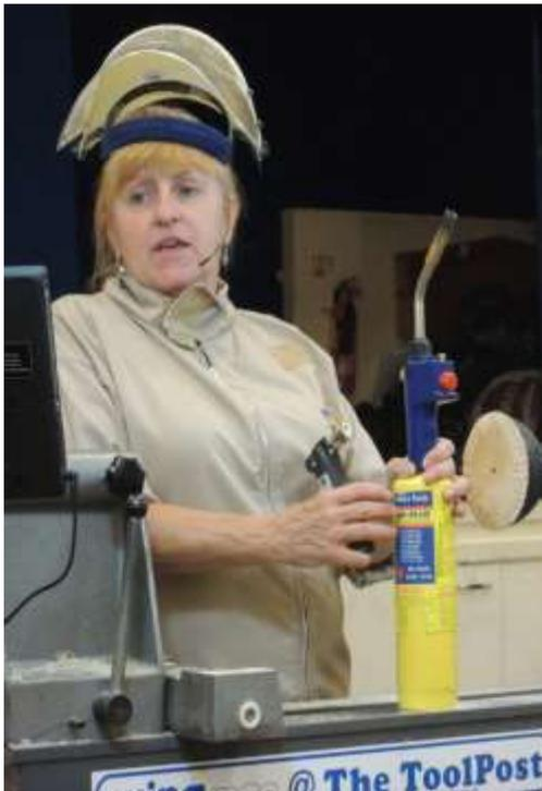
Mary used a plumber's blow torch as this burns hotter and faster. This enables her to scorch the surface without building up sufficient heat to crack the wood. Other burners are available and Mary has in the past used the small kitchen torches used to caramelize crême Brûlée, but these need to be used with care to prevent damaging the blank.
