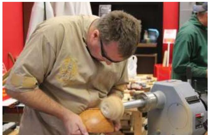
Arthur was demonstrating his way of turning wooden balls and followed by a few light pulls. To turn the balls Arthur started by roughing a small piece down to a cylinder and then using a spindle gouge turned it into two near rounds side by side as in the picture. They are then cut
