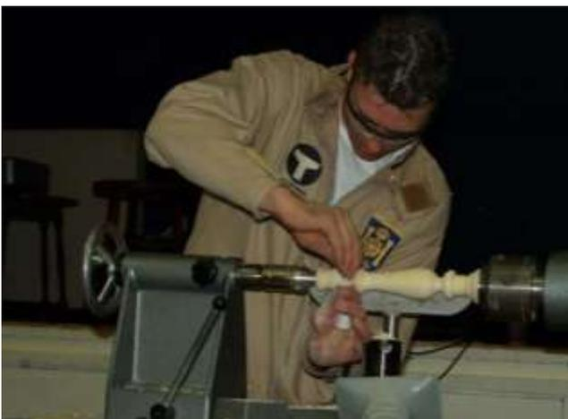
Using the Stem Design Template, Richard marked the relevant high and low points. Then using the Parting tool and a pair modified of modified Vernier Callipers he blocked out the design. From there it was just a matter of progressively defining the shape using Spindle Gouges, Beading tool and Skew.
