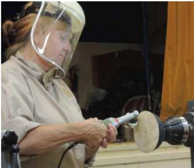
Mary mounted a previously prepared blank (more Blue Peter) onto the lathe. Then holding the cutter in both hands proceeded to make a series of cuts in the top lip of the bowl. In each case the cut was made from left to right. This ensures that the movement goes in tandem with the direction of cut, thus ensuring that the cut is always under pressure, which reduces the risk of the tool running back along the work.
