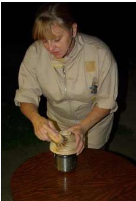
Once satisfied with the appearance the small shoulder of material left at the beginning of the process can now be turned off to create a pleasing contrast foot. (Note that the spigot remains at this stage.
