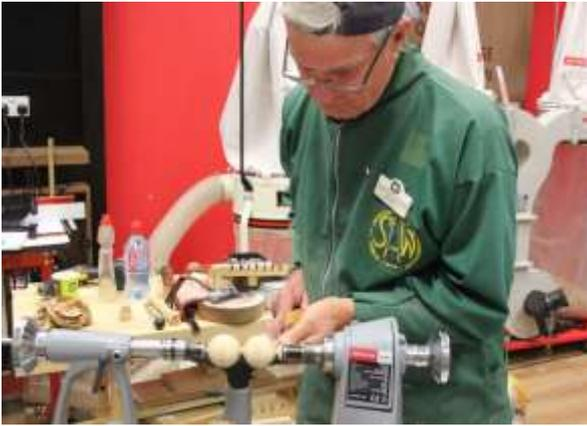
apart and each mounted between centres using what are best described as wooden cups that Arthur has made one is affixed to the drive centre and the other to a live centre. The ball is held between the cups so that the excess wood end bit can be removed and rounded, by now the ball is fairly close to the round, and so sanding can be done this removes any slight protrusions and brings it into the round. Now polishing can be done by turning the ball around between the cups until it is complete.
