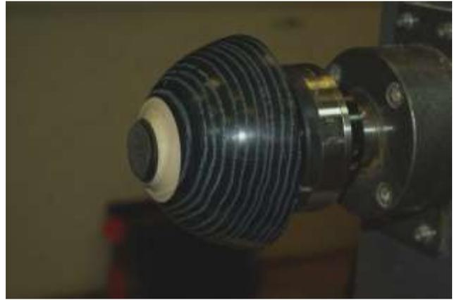
In normal circumstances the bowl would next be turned and mounted on the spigot and the central bowl area excavated and decorated as desired. The bowl would then be reversed, secured using either a jam chuck or button jaws and the spigot removed and the foot sanded to desire grit level and sealed as needed. This was not to form part of this evening's demonstration.
