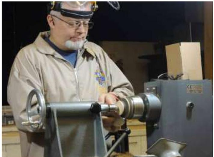
He made the pendant blank concentric then shaped the external face using the normal gouge, getting down to around 8mm thickness.
