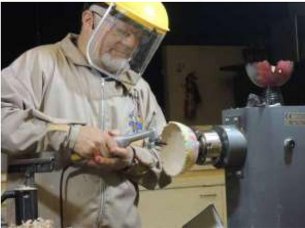
Frans then moved on to decorating the outside of the bowl. Firstly he created the faux natural edge using a mini Arbourtech cutter in a Proxon grinding tool. Then he created a false void on the piece using a battery powered Dremmel type tool.
