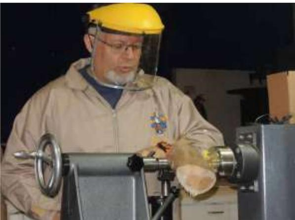
Frans used his moisture meter to check the wood, mentioning that he himself was typically 34% as a baseline to test the device and the wood was 27% which was still pretty wet. Frans reminded us to watch the shadow not the piece when turning
