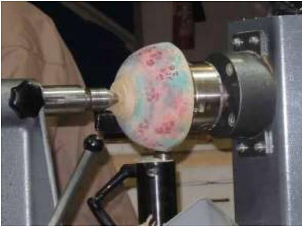
for this process and used illustrations on a notebook. This technique makes it easier to make the entering cut so you don't skip the tool across the face and allows an easier transition from cutting the side of the bowl to the bottom of the bowl.
