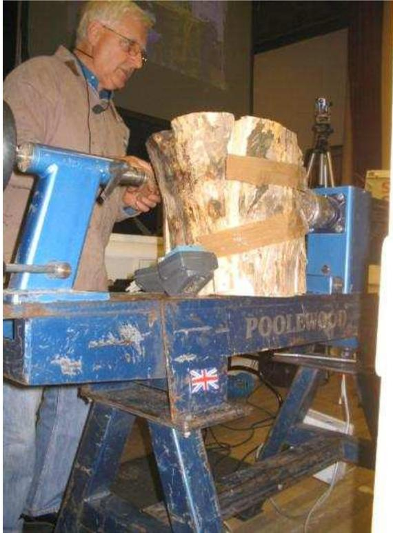
He has a selection of circular discs to draw round to give the shapes to cut on the band saw. The centre of one of the blanks was marked and this was mounted between the tail stock and the front of the chuck. He then cut a 3 3/4" spigot with a finger nail profiled gouge. The blank was mounted in the chuck jaws and the side trued up and the bottom shaped.
