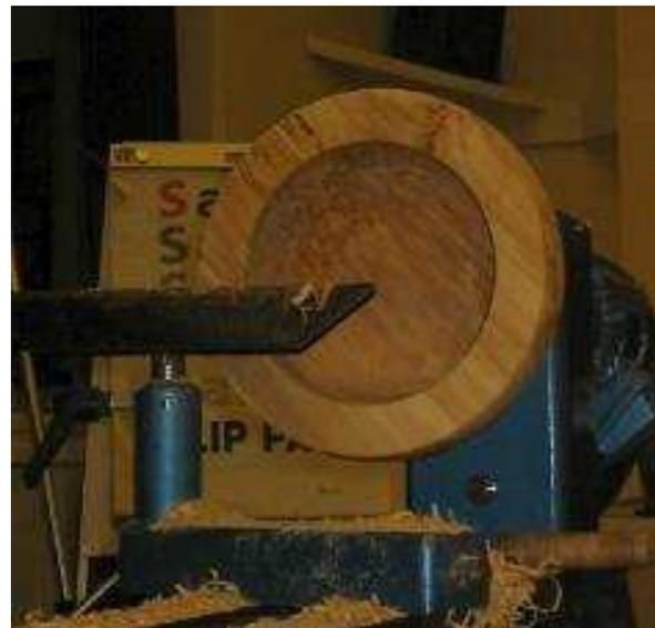
Dave had wanted to show us off centre coloured platters but time was running out, so he showed us the main principles. A blank of kiln dried Sycamore was mounted in the chuck after cutting the spigot as before. The edge was trimmed and the back shaped. The front was also trimmed, if you are going to texture you must start with a good surface. With the lathe running at slow speed a mini Arbortec was used to give the desired effect. Any hairs must be removed with coarse sand paper.
