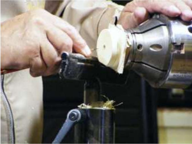
an area which almost reaches the three points of the piece. The distance remaining will, eventually form part of the final thickness of the wall.
