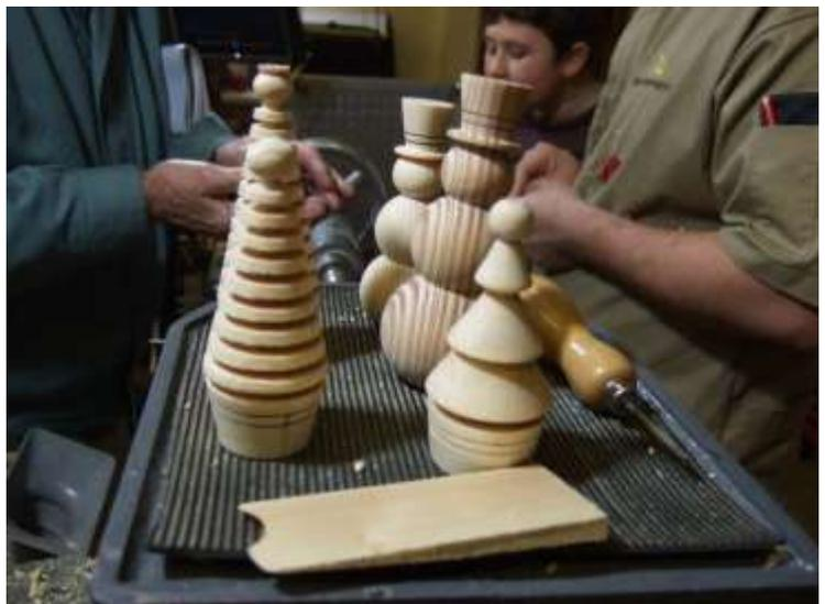
Xmas Tree Style 2 – Using a thin parting tool make a series of cuts. Start by making the first incision about a parting tools width up from the base of the tree.
