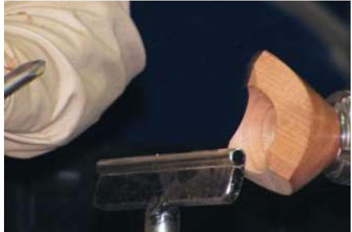
After securing the cube safely between centres test for true and rotation. Then run the lathe for a short time and observe the shadow. Stop the lathe and align the toolrest as close to the piece as possible and parallel to the tailstock end shadow. Rotate piece to ensure no catches then, standing safely to the side, start the lathe and bring speed up to approx. 1300rpm.
