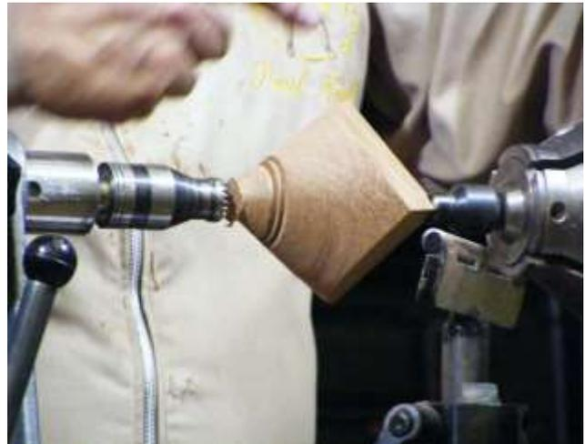
What did he need? Firstly two cubes each being perfectly square and with matching dimensions to all faces and of the same timber, plus a third piece of timber, in a contrasting colour, of approximately the same width and breadth but say a third of the depth (end grain showing on the shorter faces). Access to a good Planner/Thicknesser and/or Bandsaw an essential part of the preparation.
