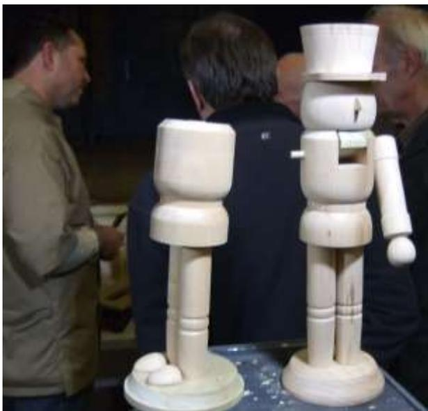
Shoes – Two pieces of stock are glued together using a paper bond. These are turned to form the shape of the shoes; the paper bond split and the heel are filed down to fit base of leg.
