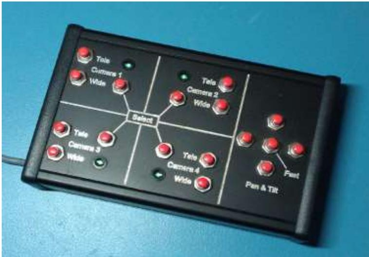
The old unit is shown here. The switches were the cheapest available, as I wasn't sure at the time how much use the unit would get when I made it. Whilst they have lasted 5 years, they have always been uncomfortable to use, as they have small tops and need a lot of push! And now they are starting to come apart, so it seems to be a good time for a change.
