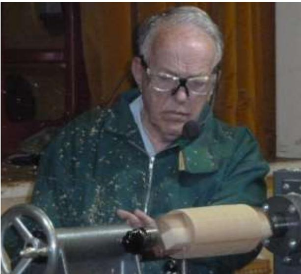
The piece was turned between a Four Prong drive and a standard Live Centre. Under normal circumstances Jim recommended that Ring Centres be used as in extreme cases it is possible that the pressure from the point of a live centre might force the block to delaminate. Members sitting in the front rows were advised to remain attentive throughout the demonstration.
