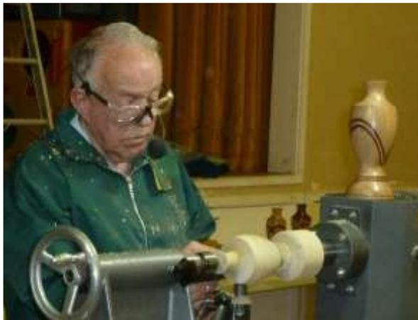
This vase was turned in the same fashion as Jim's first display. The final effect was to produce a vase with four ovoid cheeks with contrasting central core. The final finish being dependent upon the finished diameter of the vase.
