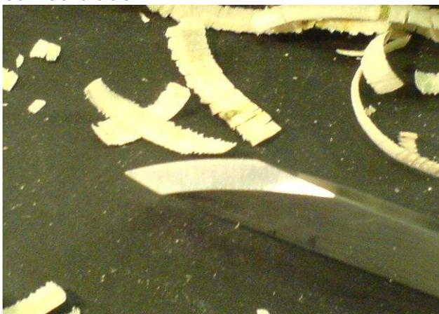
This meant it was impossible to get a dig in when using a planing cut. It was also good cutting end grain. Thus he made a tool handle.
