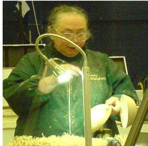
Reverse the piece in the chuck and starting from about 1cm from the outer edge start your cut. The bevel needs to be in line with your intended cut. Some people use thin parting tool to make a cut for the bevel to rub. To ensure the timber does not flex too much the middle is removed last and the thin section is turned a step at a time. Once the desired thickness has been obtained it is impossible to go back to the top edge again because it will have changed shape and will vibrate.
