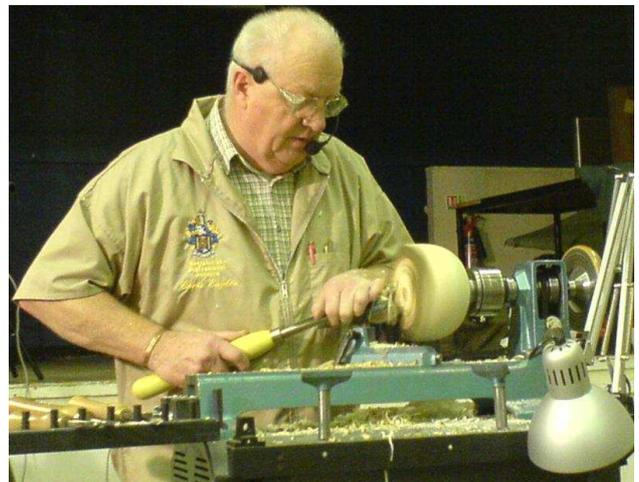
First we were shown a hook tool, then a ring tool, which is sharpened on a slip stone or card file and finally a Rolly Munroe tool which has a very controlled cut and does not clog as the shavings come out of the top of the cutting head.
