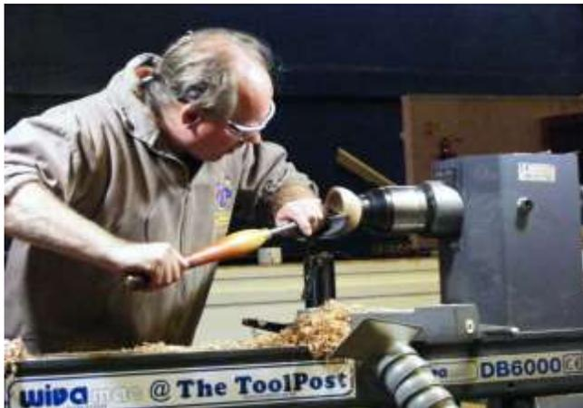
Gary then moved on to the lid, which is basically another small bowl, this time mounted on a screw chuck due to its small size. Because the lid needs to be hollowed Gary left a flat on the outside top in order to make a small spigot. He then proceeded to turn the outside bowl shape. He finished the outside with a skew chisel held close to 45 degrees to create a sheer scrape getting a very good finish in a couple of passes.
