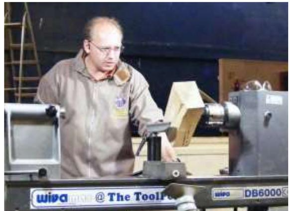
Gary likes to use faceplates and rings as they give a good fit and are quick to use, he marked the centre of the blank with a pencil and used a homemade jig to locate the ring centrally and enabling him to screw it down.
