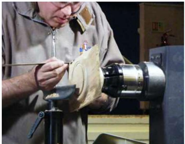
He then worked the wings down to the finished thickness, aiming for  $\frac{1}{4}$  inch as this looks nice. There was a fair amount of stopping to measure to get the thickness
