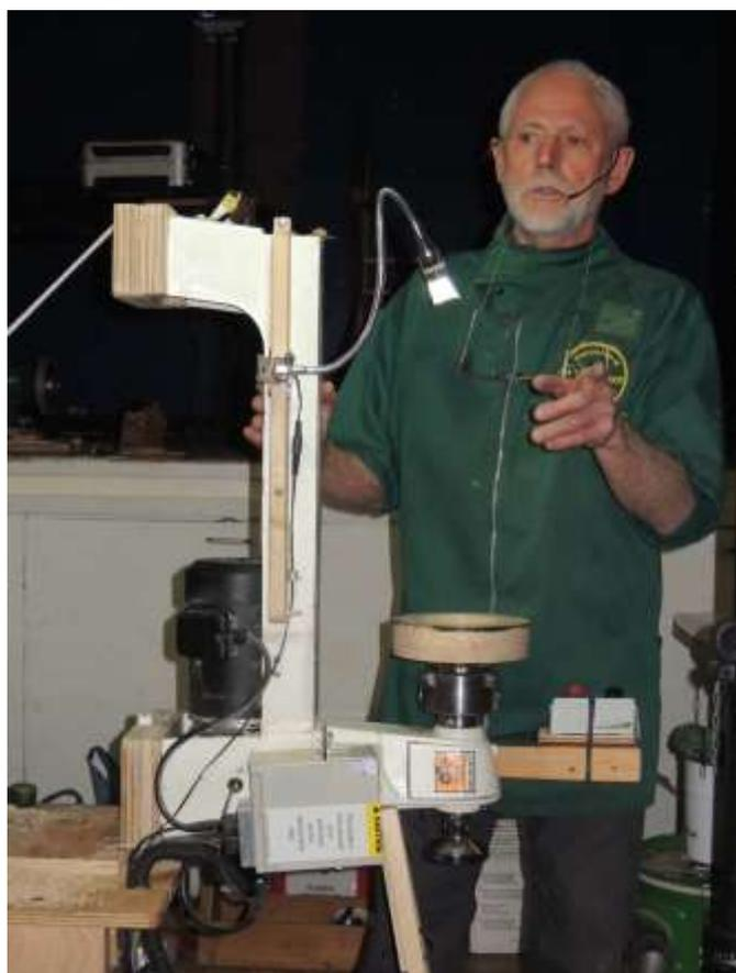
reckons 900 RPM is the ideal speed based on his experience. Due to the risks and the wood chips being removed he wore a mask and gloves. He did one quick light pass of the cutter over the surface. The result was a simple but elegant textured finish.
