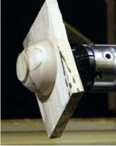
Gary notes that if you are unsure about turning with wings or it's a really big piece his suggestion is to have waste blocks added to make the blank completely round so it's safe and easy to turn and then to remove the blocks when fully finished.
