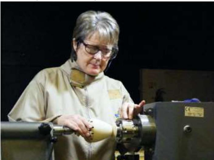
Once the outside profile is satisfactorily complete the vase is removed from the lathe and the paper joint is split, so that the insides can be hollowed out.
