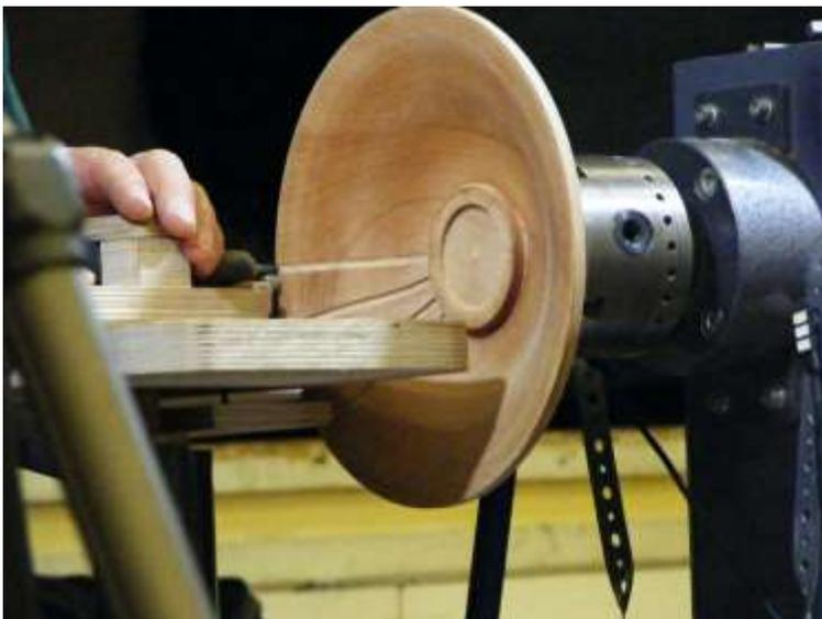
light pressure on the cradle to keep it in contact with the table. The roller bearing will enable you to stop cutting when you meet the register shoulder you have left in the centre of the piece.
