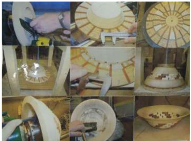
half an inch and so on to desired grade then seal and polish.
