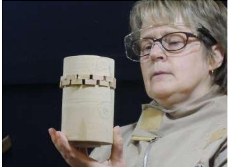
Sue used a 1/2" spindle gouge with a finger nail profile to shape the outside of the vase remembering to leave enough waste timber at the top and bottom of the vase to provide support when hollowing out later in the process.
