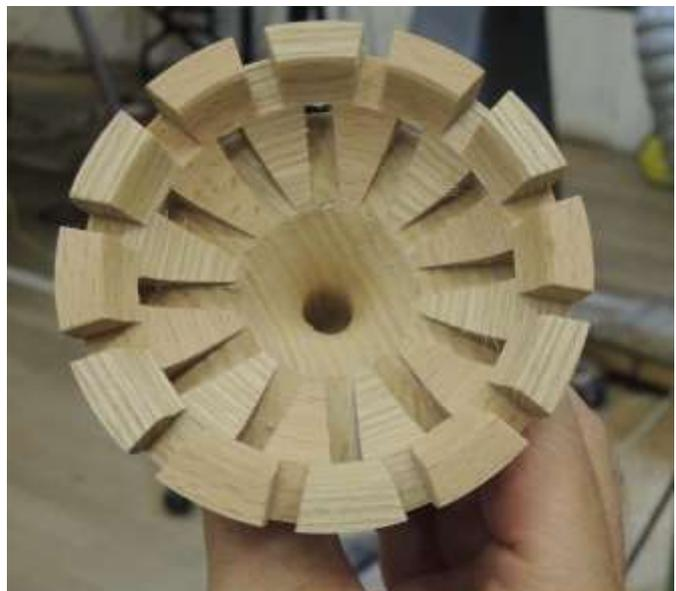
than the vase base, unless you want a drain hole in the bottom. The blank was then hollowed out. On this occasion Sue used and demonstrated a RS200 hollowing tool to remove the bulk of the material and a BCT Supercut to complete the hollowing process.
