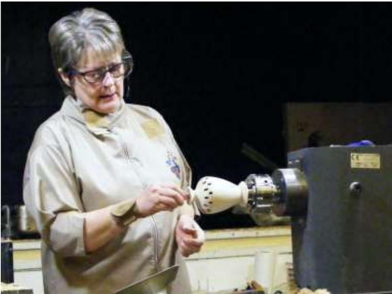
Whilst still supported by the tailstock, Sue then finished the top of the vase, shaping the inside of the top of the vase while reducing the waste wood and eventually breaking through to the hole drilled in the blank at the start of the hollowing process. Once broken through the tail stock, and more importantly the live centre can be removed and shaping of the top of the vase completed, sanded and finished
