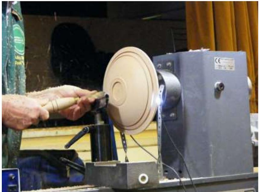
Once the second groove was completed John started to reduce the overall thickness of the platter on the outside edge and between the first and second grooves. He did this using a wider parting tool, taking small cuts and nibbling from the outside edge inward, getting down to a thickness of 3mm, John does this stage now as the platter would be too fragile to try to do this as the final stage.
