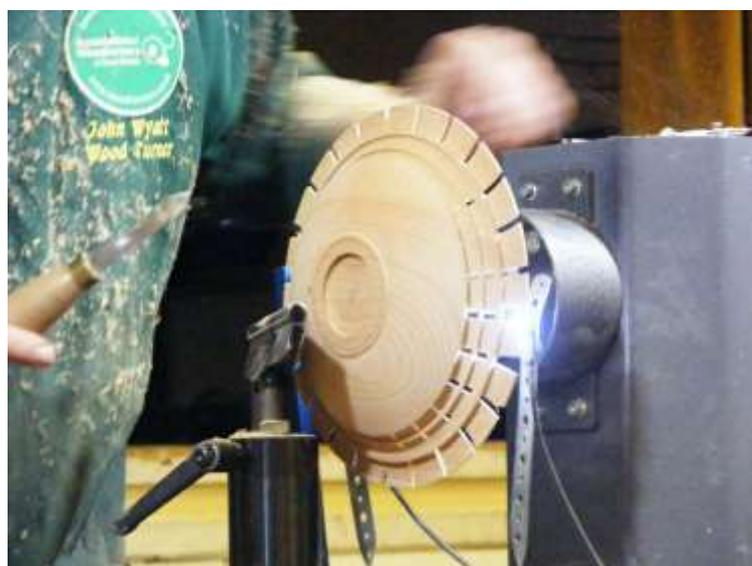
Once completed you would reverse the piece in order to remove the spigot and recess from inside the bowl and the reverse again onto button jaws to clean up the foot of the piece.
