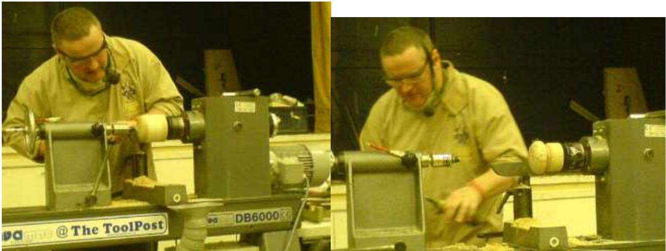
Using a gouge at 11.o'clock he started to hollow from the centre out rolling the tool to about 9.30 as he went. He then used a Simon Hope carbide tipped tool which is ideal for cutting cross grain. This he used to undercut the hollowing. A skew was used to refine the fit for the lid.
