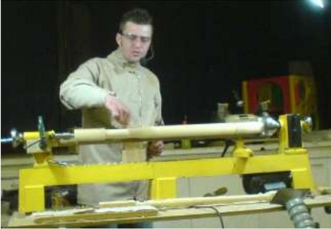
Using a slicing cut he formed the pommel at each end. Those who saw Richard the last time he came will remember his long wooden tool rest. One end fits in the banjo and the other is clamped to the side of the tail stock. He then roughed the tail end to a cylinder and using a template marked the position of the parts of the shape. On the template each mark had a small notch that a pencil would fit in to mark the wood.
