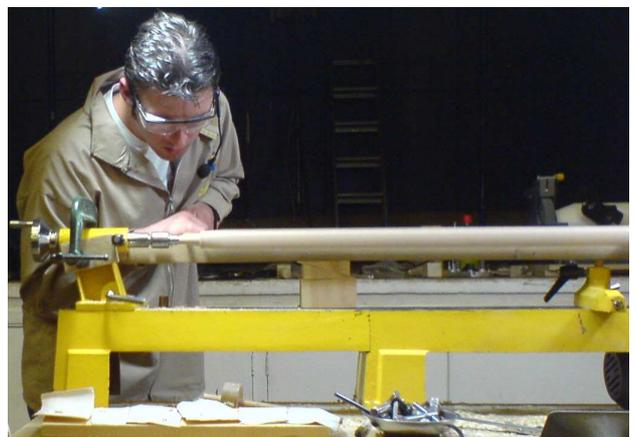
The tail fits in a ring centre. The tool rest is home made from timber. One end has a dowel to fit the tool post and the other is clamped to the tail stock with a suitable
