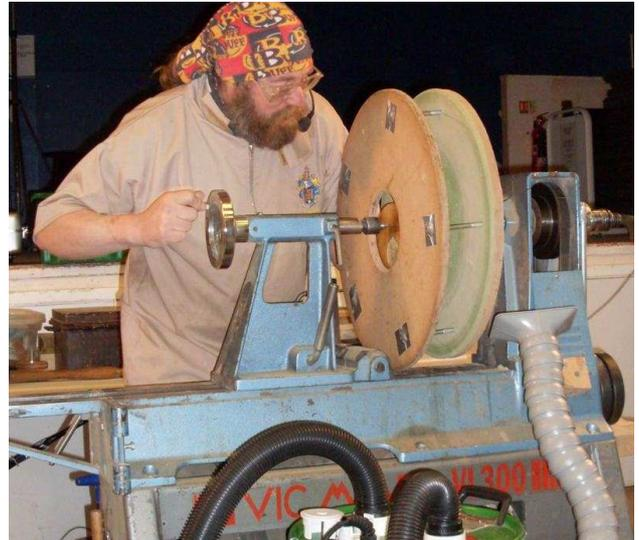
On the outboard end of the drive shaft two counter weights were fitted and adjusted to allow for the off centre bowl.
