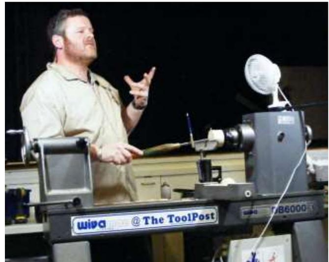
Les indicated that as he was turning end grain a better finish would be obtain by working from the centre outwards as he would be going with the grain.
