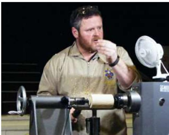
Once rounded the grain could be examined and the final orientation of the piece decided. The drive centre was removed and the chuck and jaws fitted. For tonight's demonstration Les would be using parallel jaws so no dovetailing was needed. The blanks were then fitted into the jaws using the Live Centre to ensure true line up.
