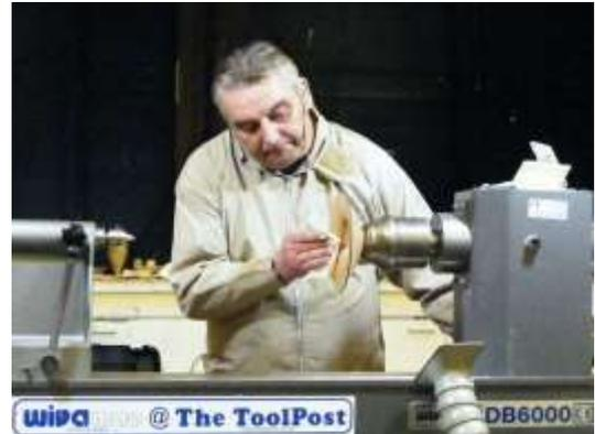
is not a safety cloth so hold it carefully so it can be pulled from your hand in a catch. Finally leave the piece for 10 minutes to let the wax harden off.
