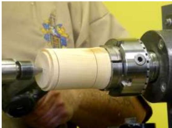
He jammed the lid back on, lined up the grain pattern and marked the final size
