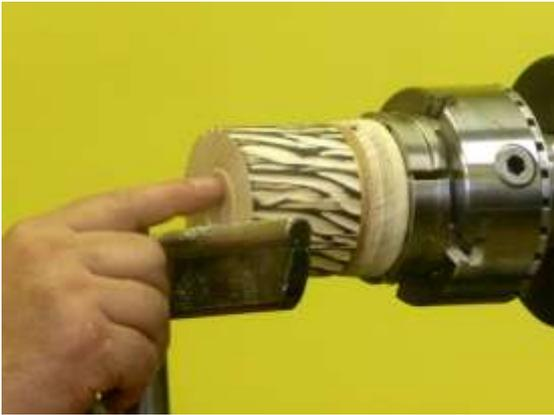
Box is reverse jam chucked and the bottom is finished. The ring is recessed
