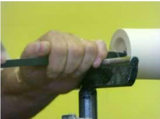
The box was hollowed out using a small carbide tipped hollowing tool
