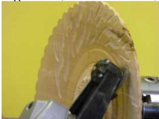
The outer part was machined with the Arbortec
