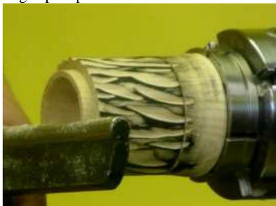
Final hollowing and polishing, then parting off
