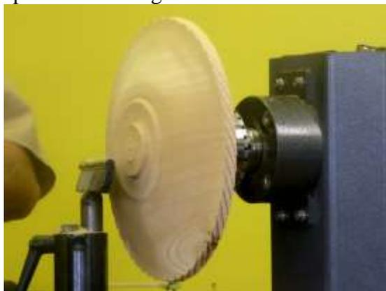
When the bottom is finished, the edge has a rippled effect (which could be coloured)
