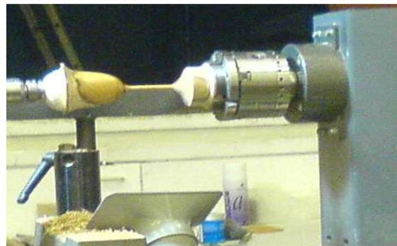
The stem was cut in 1" sections. The tail stock was fitted and a polystyrene ball used to support the bowl of the goblet.
