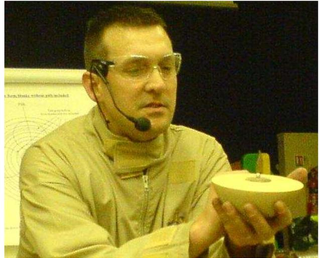
In the last 10 minutes Mark showed us an alternative made from Tulip wood. This was mounted in the chuck as before and shaped as required, A hole was made in the lid. The lid will be set into the base so a parting tool was used to form the side of the lid. This was cut off with a parting knife leaving a register mark for later. The bowl was shaped and a series of grooves cut for decoration. It would be scorched and the lid glued on. An interesting and informative evening.
