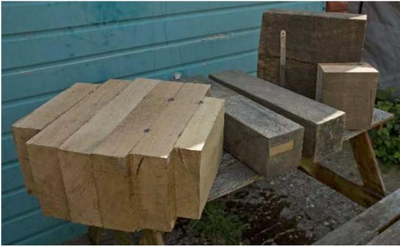
The blanks are the Base with splits on the far left, two spindles, Boss and Bowl with a 12" rule to give scale.
