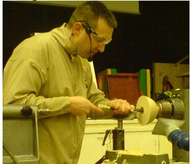
To sand inside a drill extension bit was fitted with a cut down arbour and a 240 grit pad. A wire coat hanger was bent to a suitable shape and covered with Gaffer tape. Using hook and loop tape various grades were used to hand finish inside.
