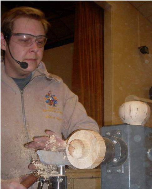
A vernier was used to measure the hole in the jar and transferred to the face of the blank. Thus a smaller cylinder was made which was a loose fit in the jar. The end was dished, decorated and sanded. This was then parted off.
