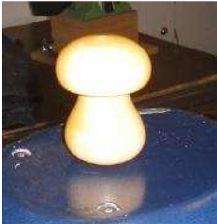
To shape the base a thread is cut in a scrap bit of wood to take the thread on the base. This is screwed on and the base shaped using small careful cuts, decorate the bottom, sand, seal and polish as before. A very entertaining evening.
