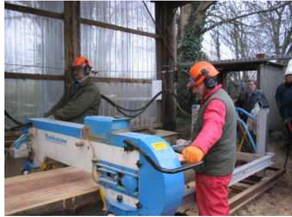
The saw requires two men to pull it along the wood as the cut is made. And two are needed to remove the planks as they are cut. A labour intensive business. Luckily John was available to lend a hand.
