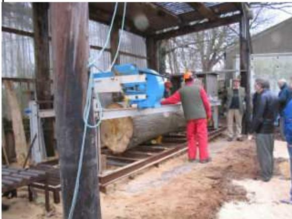
A very large band saw with a blade 4" wide is on its side supported on two guide bars which can be raised and lowered to alter the thickness of the plank. Diesel oil is used as a lubricant for the blade.
