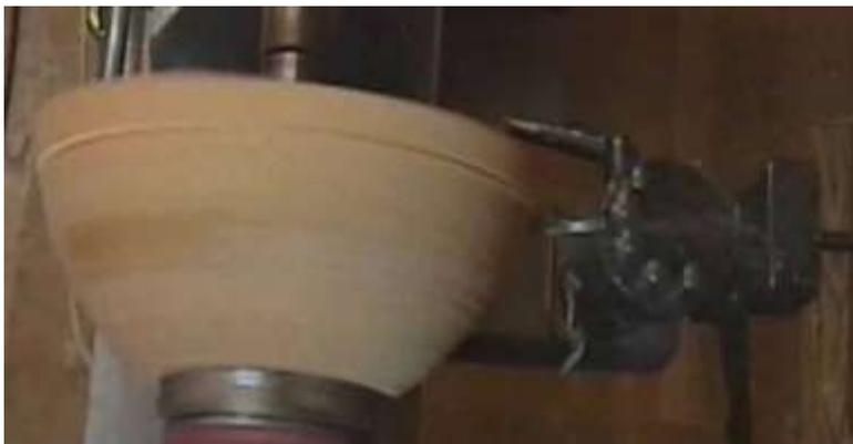
The tool is mounted in a special tool rest which restricts sideways and up and down movement taking the strain away from your wrists.
