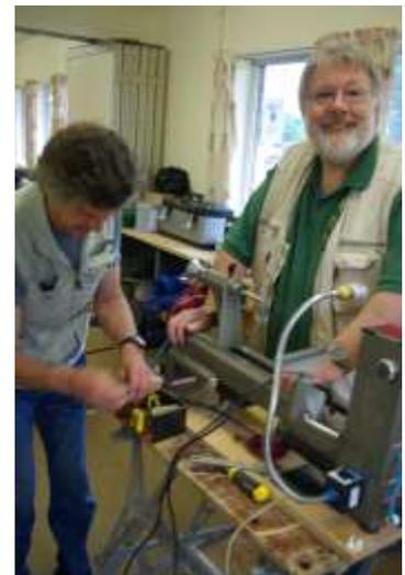
Still with a bit of juggling we got it secured between a four prong drive and a Ring Live Centre. The initial idea was to clean up the tailstock end, which was intended as the top of the bowl so that it could be fitted to a screw chuck. Unfortunately getting a suitable surface proved extremely difficult so we eventually created a spigot to fit the available jaws.
