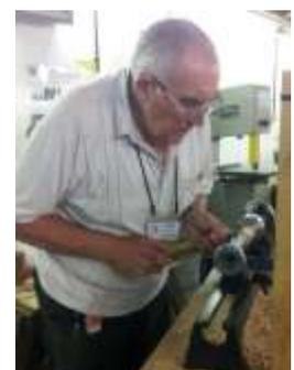
Max Bennett demonstrated a few different techniques over the weekend making a square edge bowl and a plant dibber from wild mango, a spinning top from ebony and an egg box from Purple Heart. He was practicing a technique he recently read about in the woodturning magazine using a skew chisel to take his blanks from square to round.
