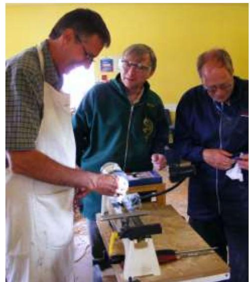
was on with the lathe and an excellent day of tuition in the use of the main tools. We covered using the skew for planing, the spindle gouge in rounding the top and discussed minimum grain loss at the joint using a thin parting tool. I tried a variety of techniques to hollow the body out, including using some specialised tools I borrowed on the day. We finished by discussing the use of abrasives and sealer to achieve a good finish.
