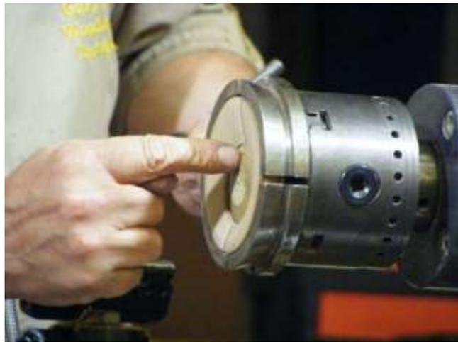
Gary then mounts the blanks into the jig, the jig is then held in the jaws of the chuck, he then drills the centre of the blank.
