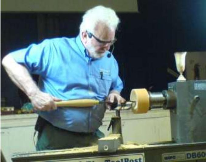
Chris Stott modified the grind on his gouge so that the left side had a longer grind. Stuart Mortimer sells 3 gouges with different lengths of flute. You need to consider the length of the tool that that will project beyond the tool rest. You should have solid bar on your side to provide the strength.
