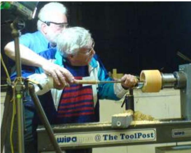
The Kelton Hook tool is far safer but is used as a ring tool. Peter Duguid got up to use it and was impressed. Sharpening is by a slip stone around the outer edge.
