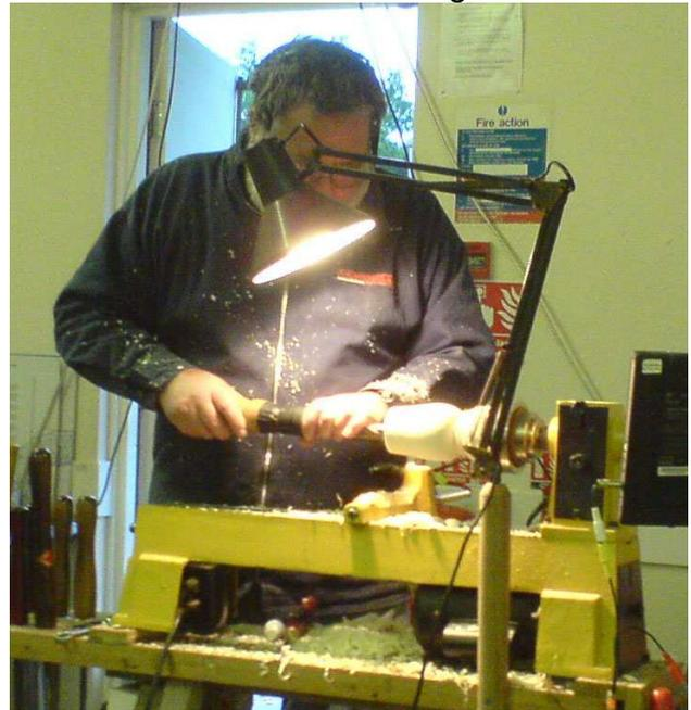
Bill then went on to demonstrate his laser guide hollowing apparatus. The cutting element was a 19mm round steel bar drilled at the end to accept a cutting tip from Axminster held in place by a grub screw. This fitted into a framework with another bar above, at the end of which was a laser. The laser came from Maplin and was powered by 5 volts generated by part of an old PC.
