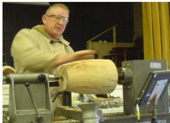
Tony used the club lathe and mounted a 12" X 9" dia. Spalted Beech log between centres. Using a large roughing gouge he started to shape the end. Then using a swept back bowl gouge he cleaned up the base and cut a spigot for the Axminster chuck.
