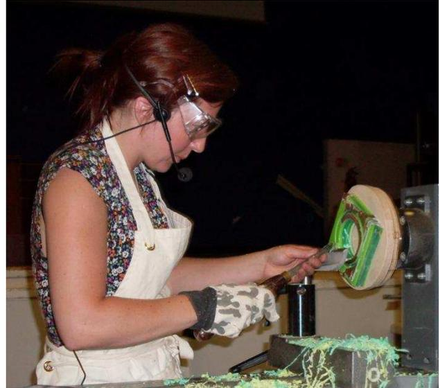
Several sheets of light and dark green acrylic had been glued together and then screwed at the corners on to a ply disc which had been screwed on to the face plate. Using a parting tool Sarah proceeded to cut out the centre. She wears a glove on her right hand as some bits of acrylic can hurt as they come off the lathe. The inside was trimmed and sanded. She uses wet & dry down to 400 grit. Then Teflon Mirror Glaze or Plastimax polish from Axminster was used to polish the inside.
