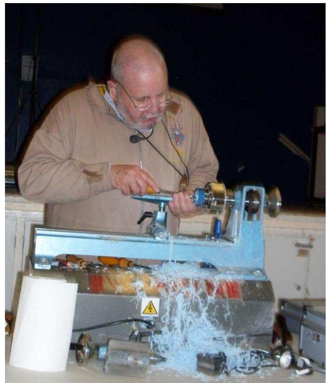
A recess was cut inside at the back and a chamfer created at the front. The inside was then polished with BGF cream. This Bloody Good Finishing cream comes in two bottles. Use the white first and then the
