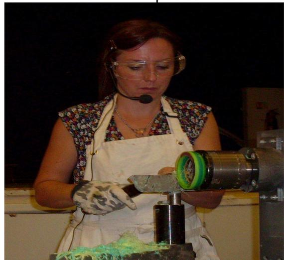
Using the parting tool again the bangle was cut out of the block. This was held by a thick elastic band around a home made chuck used in an expansion mode. With a spindle gouge the outside was shaped, sanded and polished. The bangle was reversed on the chuck to clean, sand and polish the other edge. Sarah can sell a bangle for £60.00.
