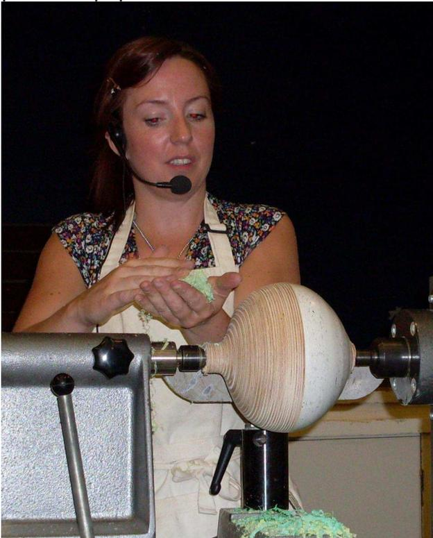
Apparently it takes a long time for the glued paper to dry. This was shaped with a spindle gouge. Then sanded and polished. Sarah also showed us how easy it was to cut a leather block. The tools need frequent sharpening otherwise the acrylic will shatter.
