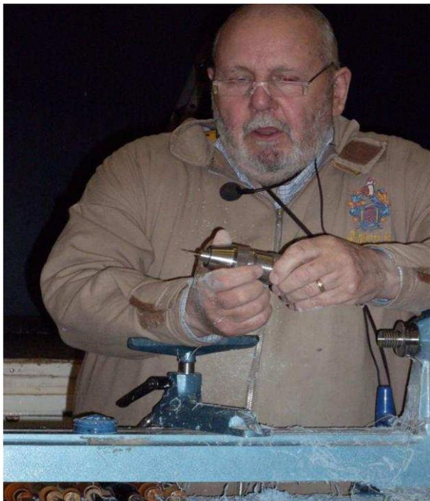
John showed us a rotary chisel that he had bought. With this fitted in a Dremmel he made a series of scollops around the edge of the lid. A doctored nail head was also used to decorate the top, which was then polished. Silver gilt cream was used to enhance the effect.
