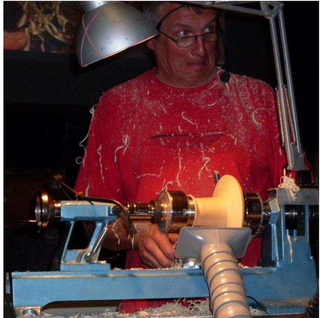
Because this hat is only going to be 1mm thick Phil had to constantly re sharpen his gouges using a jig on the grind stone. The points of the callipers had been rounded off to ensure there was no damage when checking measurements.
