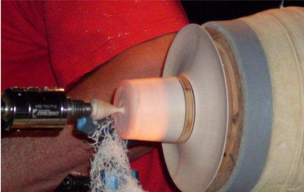
To form the hat band a thin piece of Ebony and a piece of Rosewood were cut across the end at an angle and applied to the revolving hat so that the friction caused the colour to be transferred.
