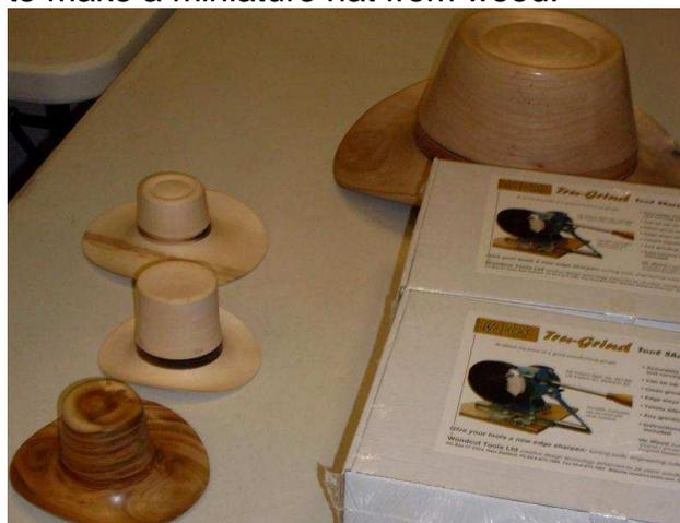
He explained in detail the process of making a full size hat. The grain must be straight, running front to back and can be from a variety of wet timbers, Maple, Silver Birch, Sycamore, Oak and London Plane. Elm is not recommended. It will take four
