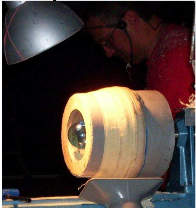
He has made a special jamb chuck in the form of a large cylinder with suitable padding on to which his full size hats could fit. This had a light bulb in the middle with the power lead running through the head stock. On the end of this was secured the wooden mandrel from which the internal dimensions of this hat had been taken.
