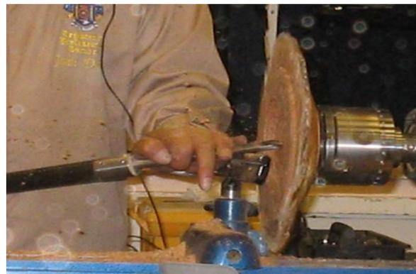
He switched to a ¼" bowl gouge and then another 3/8" bowl gouge where the bevel was a lot less but the wings ground down. This allowed him to cut the dish quite shallow. More power sanding removed the pimple etc. The inside was then oiled and buffed.
