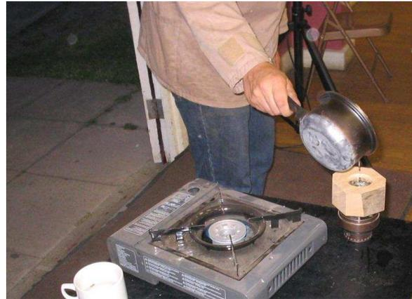
It does not require much heat. I have made fishing weights and model ship fittings in lead, so I know how easy it is to use such a material. Be careful when cooling the mould if you pour water on the hot pewter it will spit steam at you. Simon used a wet cloth.
