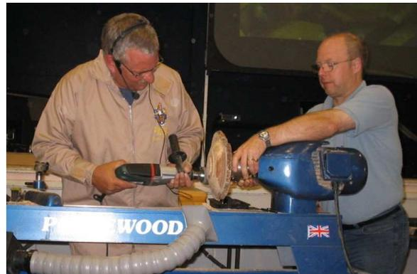
A coat of Danish oil was applied and given a minute to dry before being buffed with paper towel.
