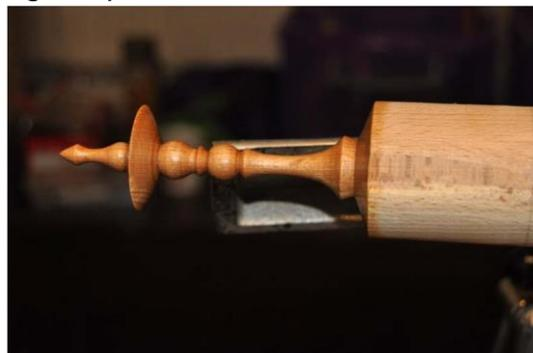
The bottom finial was produced using sharp tools, Emma used a bowl gouge to do some of the horse work, removing material and swapped to the spindle gouge to refine the shapes. Emma spoke about ensuring that you do not get any hooks on the gouge wings when sharpening as this can cause catches. The finial had a series of flat disks along it as well as lovely fine points, Emma said that she makes them like this to balance out the overall bauble.
