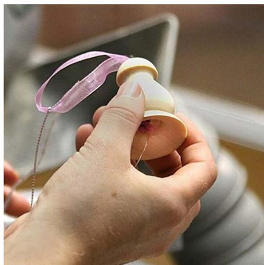
With the remaining 1/3<sup>rd</sup> of the timber Emma started by hollowing out the shape of the bauble including its neck, making sure that the hole was slightly over-sized for the neck so that any movement of the timber would not shatter the glass bauble. She then drilled in using a 4mm drill in the Jacobs chuck to create the hole for the lights and wire to go through, you may need a
