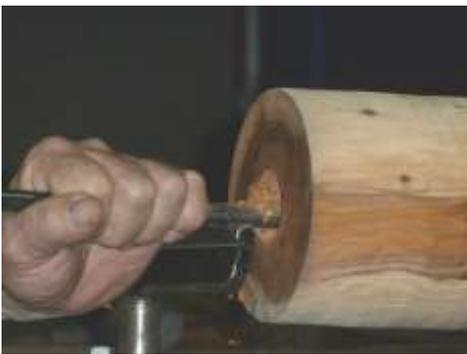
Paul set up the spindle blank using the hollow drive from the kit at the tail stock end and a normal drive at the headstock end. He did
